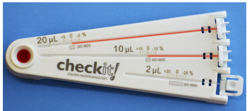
Checkit evaluates a pipette at the top, middle, and bottom of its range.
