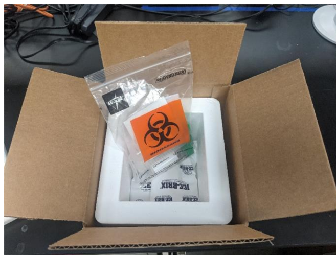
Figure 3. Fully assembled sample collection kit to be provided to wastewater utility prior to sample collection. Collection kits should be provided with a return shipping label (not shown).
