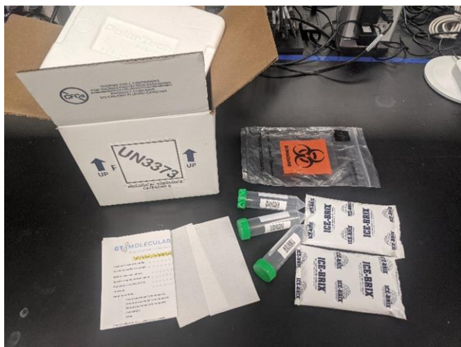
Figure 2. Individual components suggested for assembly of a sample collection kit, including 3 x 50 mL conical tubes, 2 absorbent sheets, 1 biohazard bag (with document pouch), 2 ice packs, a Chain of Custody form, 1 UN3373 sticker, 1 styrofoam shipping cooler.
