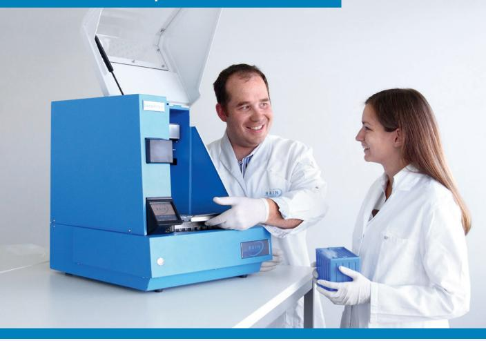
**GenoXtract**® is an instrument for the efficient extraction of nucleic acids from various sample materials. Based on "magnetic bead technology" processing of 1 – 12 samples is possible harbouring a minimal risk of contamination. Ready-to-use reagent cartridges promote flexible and reliable processing.
